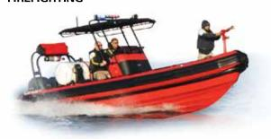
100% Customizable as per the needs of any assignment, our firefighting boats are capable of pumping 1325L/min at 10 bar pressure and 3m lift. They provide more pumping capacity than any other firefighting RIB of its size. The monitor rotates 360 degrees and has a vertical movement of 90 to 45 degree horizontal with a reach of up to 20m.
